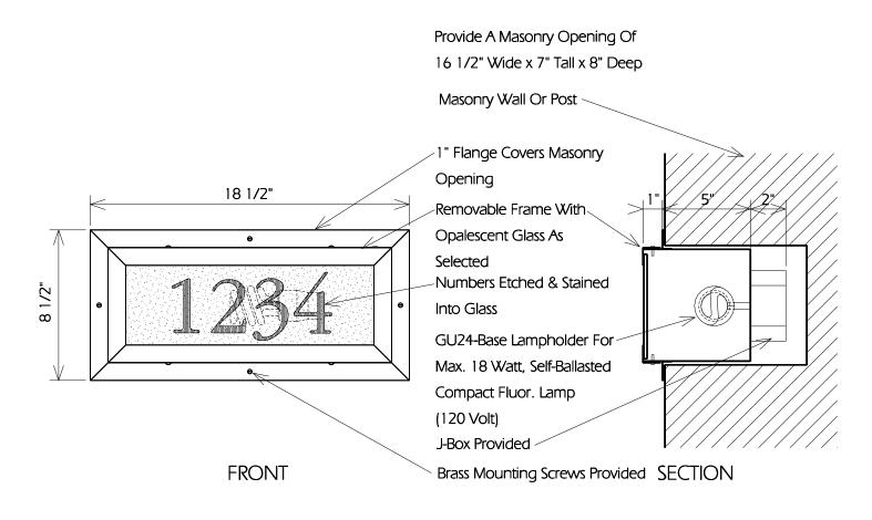
This Fixture Is Only For Installation Into A Masonry Wall Or Post
